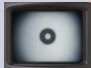
FT600 FiberInspector Pro (250x) shows clear image of multimode fiber end-face ferrule
