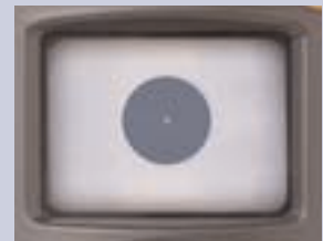
FT600 FiberInspector Pro (400x) shows higher magnification image of singlemode fiber end-face
