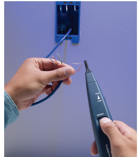
Hear the tone change when you short the correct pair on the far end
